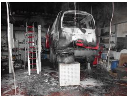
Consequences of incorrect LPG recovery
