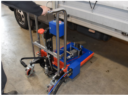
Simple tank connection for fuel removal
